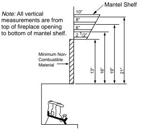
Figure 9 - Minimum Mantel Clearances for Built-In Installation
